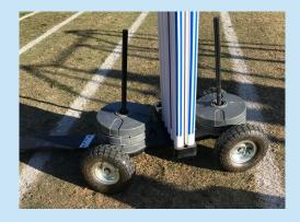
It is very important to ensure that the weighted bases are evenly placed on the trolleys, with more weight towards the front (where the trolley handle is). Failure to do this can result in the trolley tipping up whilst taking it up the path and damage the equipment.
